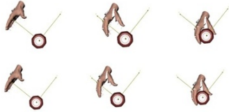
Fig. 10. On the top figure snapshots of the trajectory conducted by the human during grasping a bottle are depicted. On the bottom figure snapshots of the simulated hand following the trajectory generated by the proposed control law during grasping a bottle are depicted. In this figure the top view of the grasping experiments is depicted.
