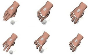
Fig. 8. On the top figure snapshots of the trajectory conducted by the human during grasping a glass are depicted. On the bottom figure snapshots of the simulated hand following the trajectory generated by the proposed control law during grasping a glass are depicted. In this figure the top view of the grasping experiments is depicted.
